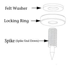
Figure 10: Combination Spike/Glide Detail
