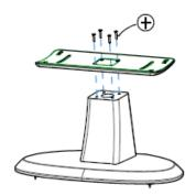
Step 6: Use the four Phillips head screws located in the Pedestal accessories bag to install the cradle to the top of the Voice2 pedestal. Tighten the screws firmly but do NOT over-tighten.
