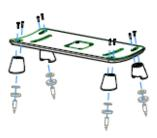
Step 3: If the combination spikes/glides were installed on the cradle, remove the spikes, felt washers, and knurled locking rings. If the combination spikes/glides were not installed, continue to Step 4.
