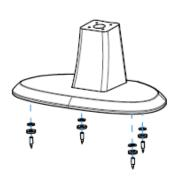
Step 5: Install the combination spikes/glides with the felt washers and knurled locking rings to the bottom of the Voice2 pedestal. Hand-tighten the spikes firmly, but do NOT over-tighten.
