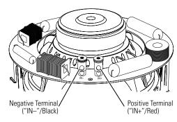
Press down on the top of the terminal to open the hole; insert the bare end of the wire into the hole; and release the terminal to secure the wire.
