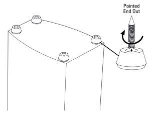
If you wish you can install the spikes with the pointed ends protruding from the cabinet for placement on wood, linoleum or tile floors. In this case you must place coins or similar items under the spikes to avoid damaging the floor surface.
