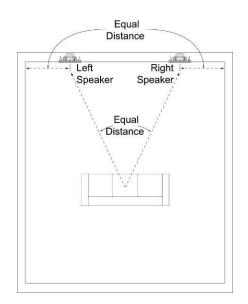
Place the left and right loudspeakers the same distance from the primary listening area (or as close to the same distance as possible).
