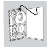
5. Connect the speaker wire from the amplifier to the speaker as explained in "Making Connects".
