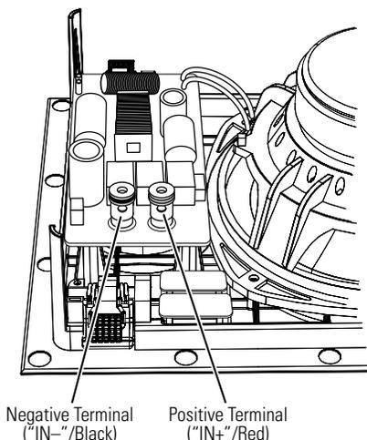
Press down on the top of the terminal to open the hole; insert the bare end of the wire into the hole; and release the terminal to secure the wire.
