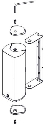
Figure 7 shows the supplied wall mount end caps fitting over the ends of the wall bracket, and then re-secured by the screws fitting through the threaded insert holes using the hex wrench.
