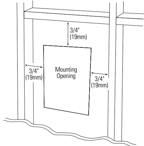
2. Determine the correct speaker location and use the template included with the speaker to mark the wall material.
