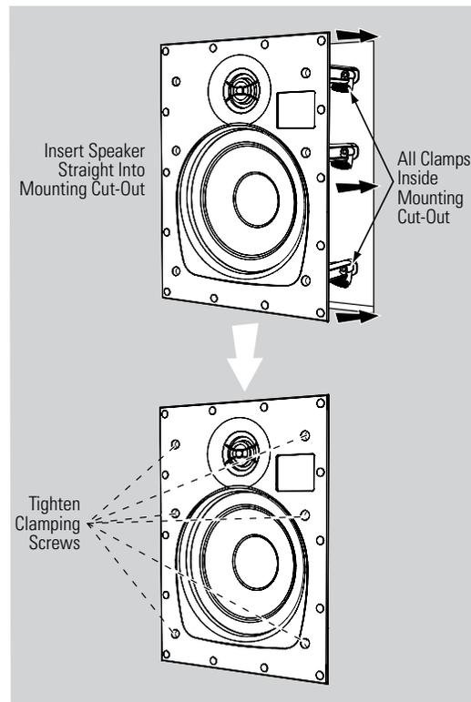
**IMPORTANT: Always use low-torque settings. NEVER over-tighten the clamp screws.**
