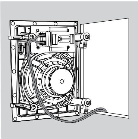
5. Make sure all of the speaker clamps are retracted in their “ready-to-mount” position at the tops of the mount towers, tucked within the mounting opening’s border.
