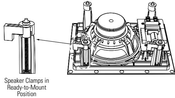
6. Insert the speaker straight into the mounting opening. Tighten the speaker clamp screws on the front of the speaker baffle. The speaker clamps will automatically rotate into position and begin clamping the speaker.
