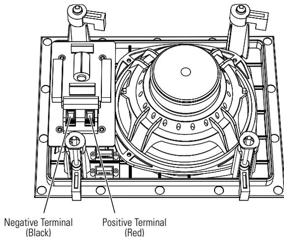
Press down on the terminal's tab to open the hole; insert the bare end of the wire into the hole; and release the tab to secure the wire.
