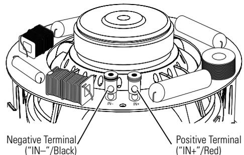
Press down on the top of the terminal to open the hole; insert the bare end of the wire into the hole; and release the terminal to secure the wire.
