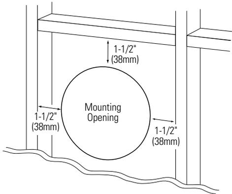
2. Determine the correct speaker location and use the template included with the speaker to mark the ceiling material.
