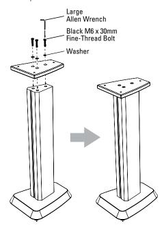
4. Attach the speaker to the stand as shown in the illustration below. Only Revel Performa3 M106 and M105 speakers can be attached to the M-Stand. Use the VELCRO® strap on the rear of the stand for wire management.
