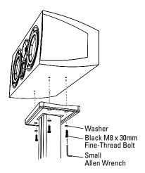
IMPORTANT: If you are attaching the C208 or C205 to the C-Stand you cannot use the adjustable feet that were included with the speaker. The C-Stand places the speaker at the proper angle for seated listeners without requiring additional adjustments.
