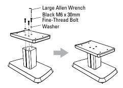
4. Attach the speaker to the stand as shown in the illustration below. Only Revel Performa3 C208 and C205 speakers can be attached to the C-Stand.
