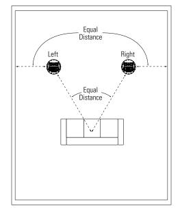
Ideally, the distance between the left and right loudspeakers should be slightly less than their distance from the primary listening area.
