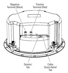
Press down on the top of the terminal to open the hole; insert the bare end of the wire into the hole; and release the terminal to secure the wire.
